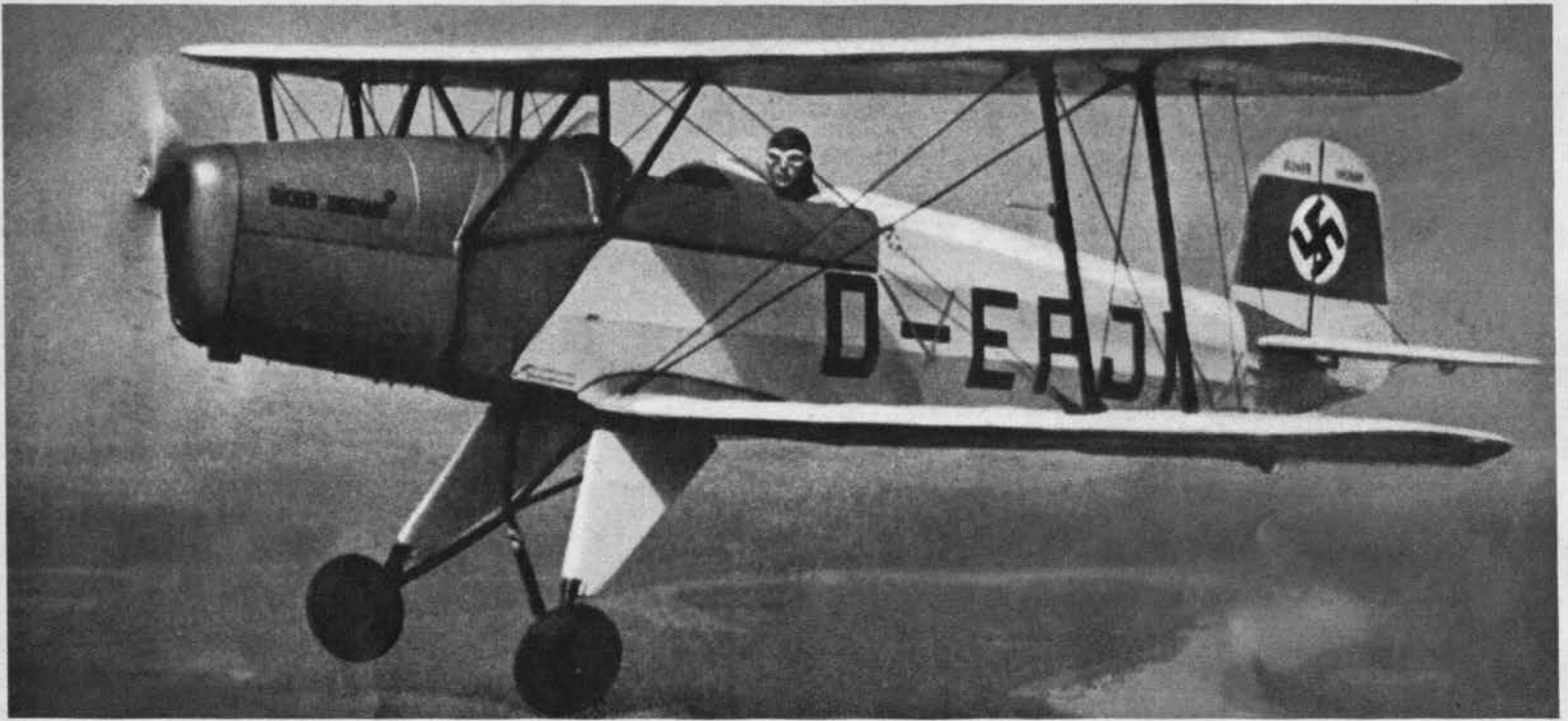
Cypress , a primary trainer used by both army and navy, was originally a German design. First built by Bücker Jungmann, it is a small two-seat
